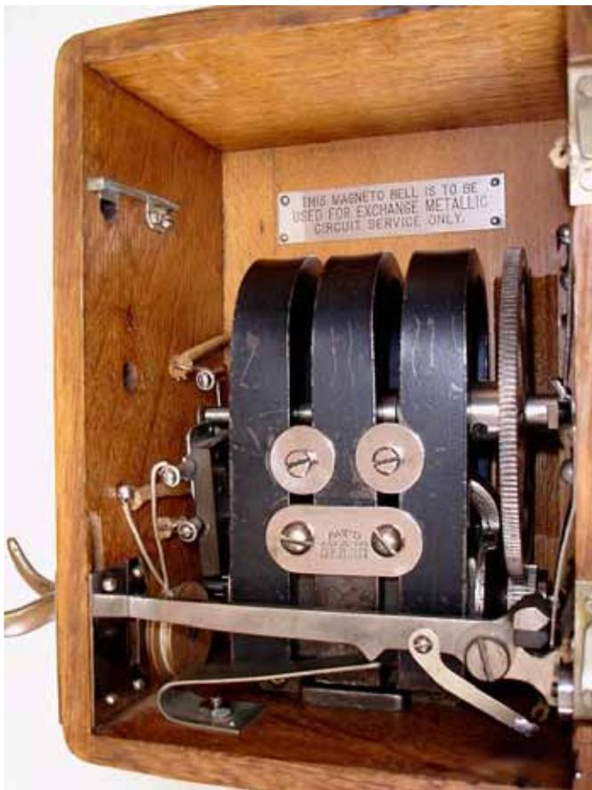
The ringers on the mag boxes were 1000 Ohm, 1517 & 1518A ringers with full nickel plate with long ringer mounts. The binding posts were the mid 1890's knurled ring style again sporting a little more nickel plating and fancy knurled workmanship.
