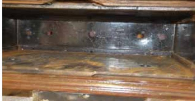
I was able to slip a small mirror into a slot in the box, hold a small mag light and hold a long shaft screw driver ( a pretty good trick since I only have two hands). Once I removed the four screws the lock fell back and drawer slid open. It was off to Bob's shop for the necessary repairs.
