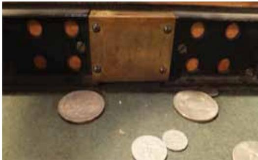
This last photo is of my restored Gray #2 Silver dollar pay station. Even though I had to drill two quarter inch screws into the cash box it was necessary in order to open the box, repair the lock and have keys made, with the backboard in place the holes are not visible.
