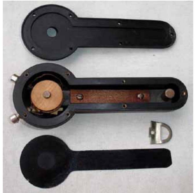
The switch hook assembly in this phone is covered by Patent No. 571,162. It is unusual and was to be manually operated by hand. The receiver hook itself serves no purpose other than a place to hang the receiver and lock the switch in place when in the talk position.
