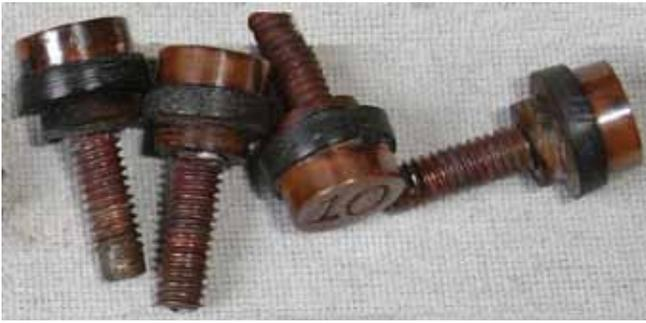
Individual station numbers (shown on left) show the copper flashing covering the threads.
