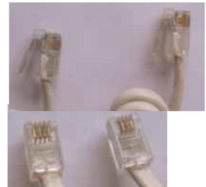
Cord Type #11—One piece small clear plastic plug same on both ends; small copper blades; WE molded on plastic clips; a) color conductors, b) black conductors, c) silver conductors; Modular cord, code changed to H4DU.
