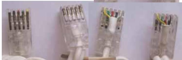
Cord Type #9—One piece tapered clear plastic shell, clip and grommet; one piece square clear plastic shell, clip and grommet; base metal tips; no stamping on clips; silver conductors, metal clamp; flat cord.
