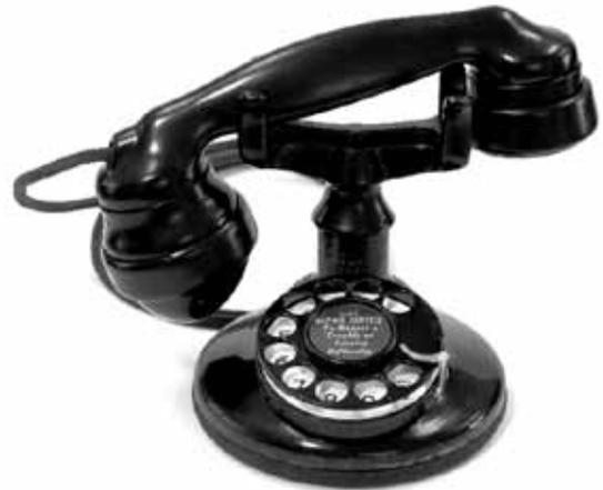
Fig. 2. A-type desk stand showing the "receiver-off-hook" (ROH) design flaw.
