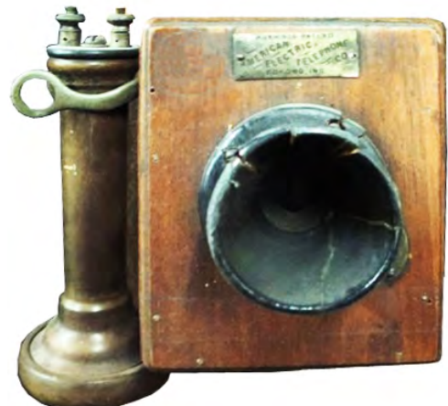
On the right is an American Electric Co phone with a Hunnings Patented transmitter.
