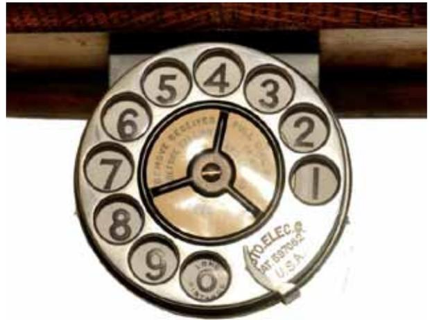
A view of the inside of the phone. It appears as the celluloid connecting plate was added to accommodate the dial adaptation.
