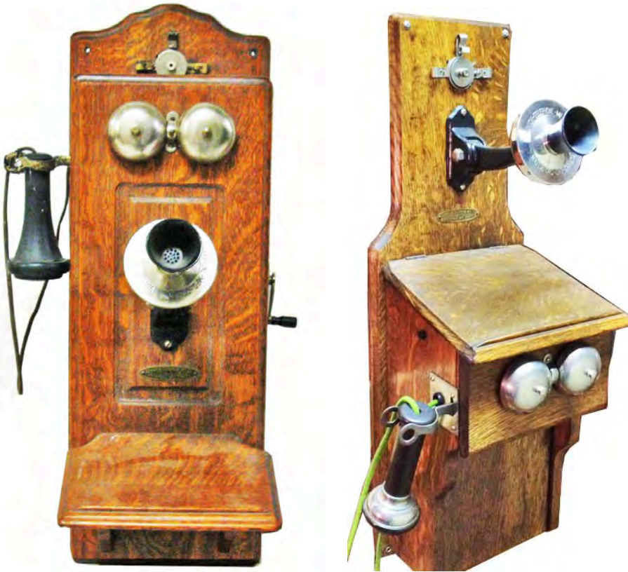
Note typical Swedish American transmitter mount on this PFFCT. Dominion made both the cast and pressed steel arms
